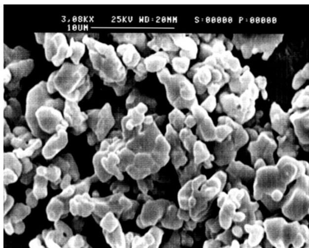
Fig. 5 SEM photograph of YNbO 4 :Bi particles.
